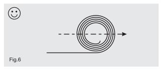
A cable bundle always shall be layed straight, to prevent a possible blocking during the installation. If e.g. several cables are layed parallely in cable trays, it is recommended to bundle them with cable straps or insulating tapes (fig.7).
